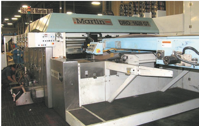
A Martin 3-color 1628 DRO GT rotary diecutter was one of two new purchases of Martin machinery for President Container's Super Plant. The company rebuilt their six other Martin flexos prior to their installation.
